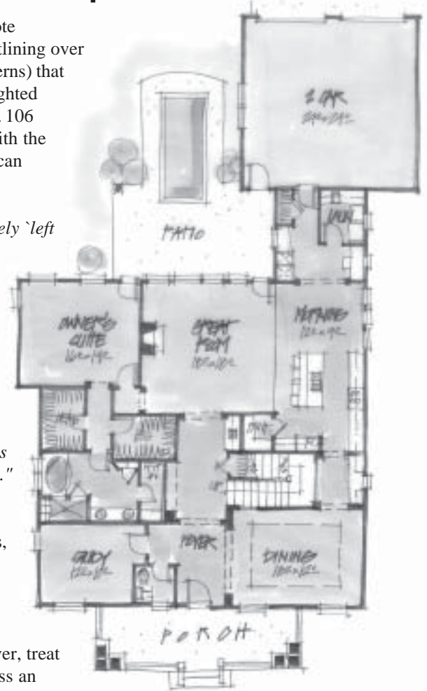
The rear loaded garage and connecting wing define the outdoor patio space and give it a sense of enclosure. Floor plan by David Court.
